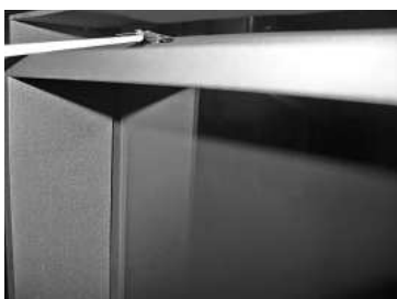
- With the hook, pull the thin, metal spring strip on the top middle from the stud on the frame.
