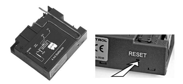
Figure 3: Receiver "RESET" button
