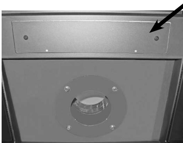
Check functioning of overpressure hatch.
