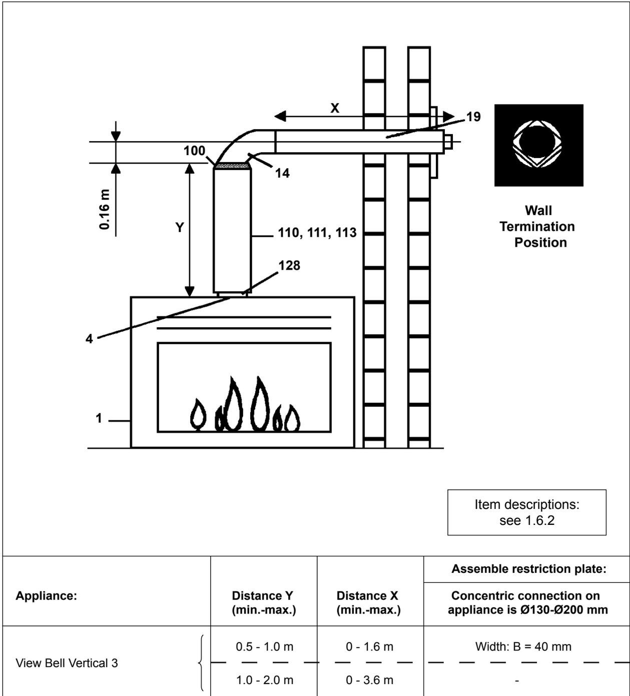
**Figure 11: Horizontal wall termination**
