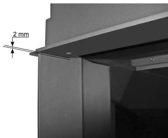
Ensure that the height between the mantle iron and the underside of the glass is the same at left, middle and right.
