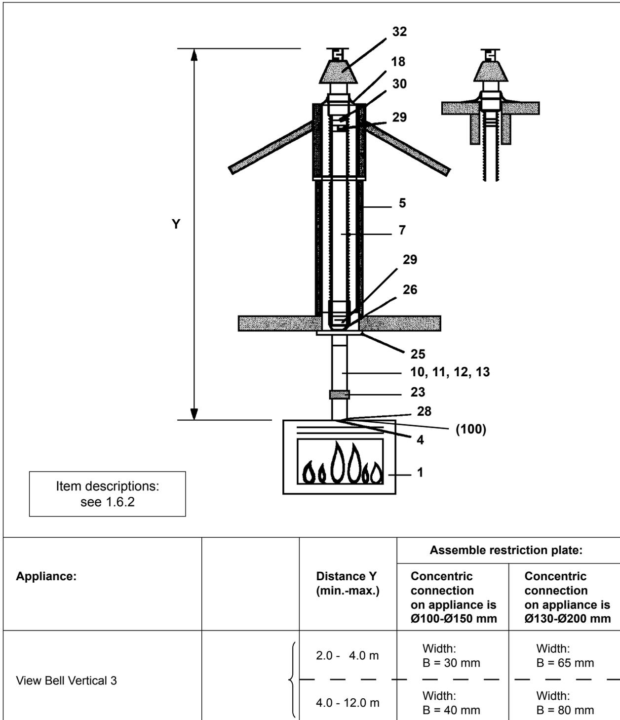
**Figure 6: Vertical chimney outlet using an existing lined chimney**
