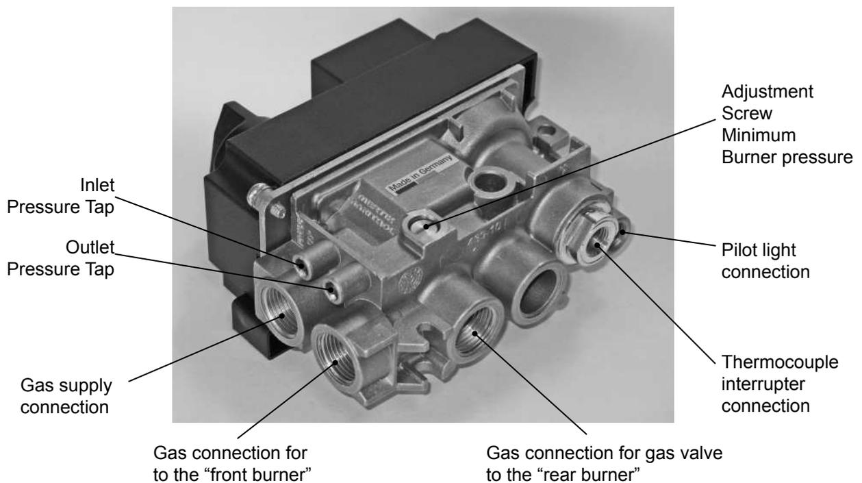
**Figure 25: Gas regulator block - Rear**
