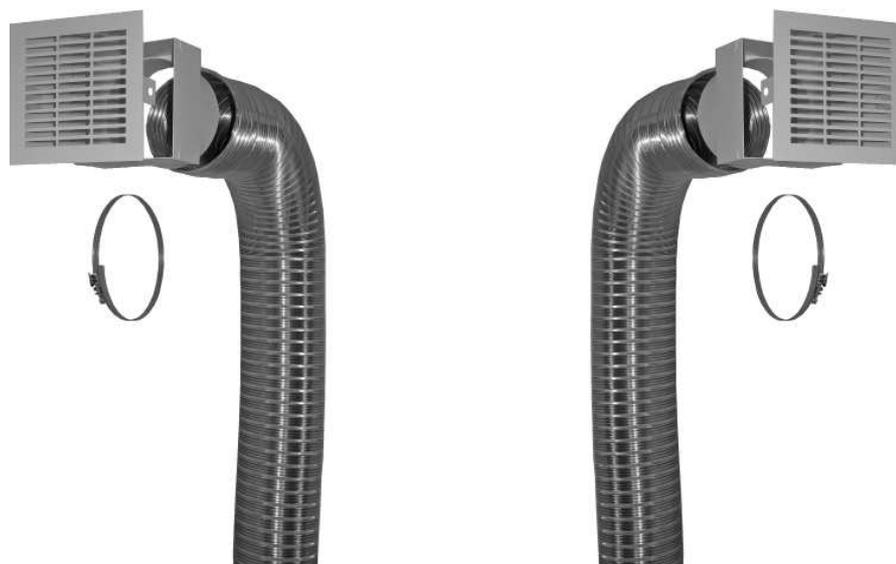
Position the two fitting boxes in the fireplace/cove, at a minimum distance of 30 cm under the ceiling. Mount the other end of the aluminium pipes onto the fitting boxes. To do this use the hose clamps supplied. When the fireplace is completely finished, mount the grilles onto the fitting boxes.
