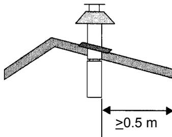
**Figure 1: Roof-mounted outlet**
