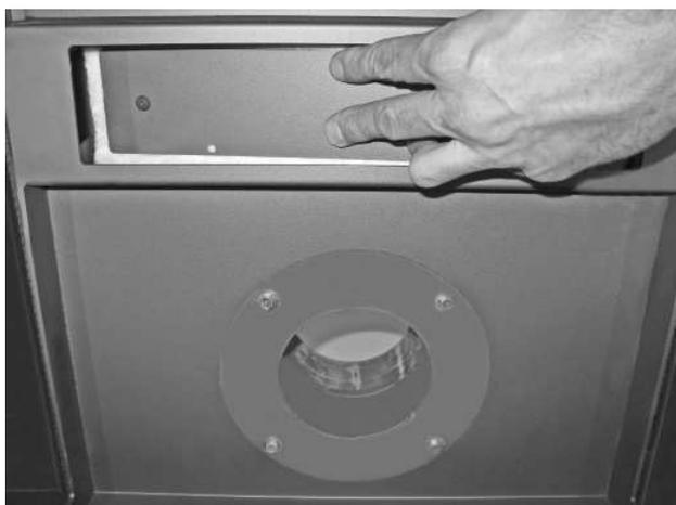
Check packing of overpressure hatch.
