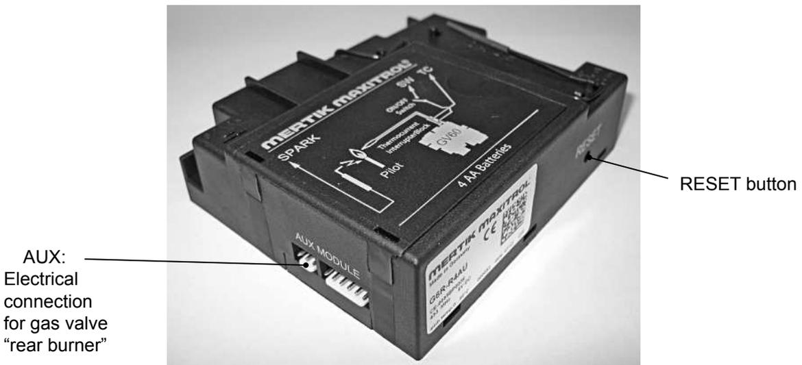
Figure 27: Receiver - AUX connection - RESET button
