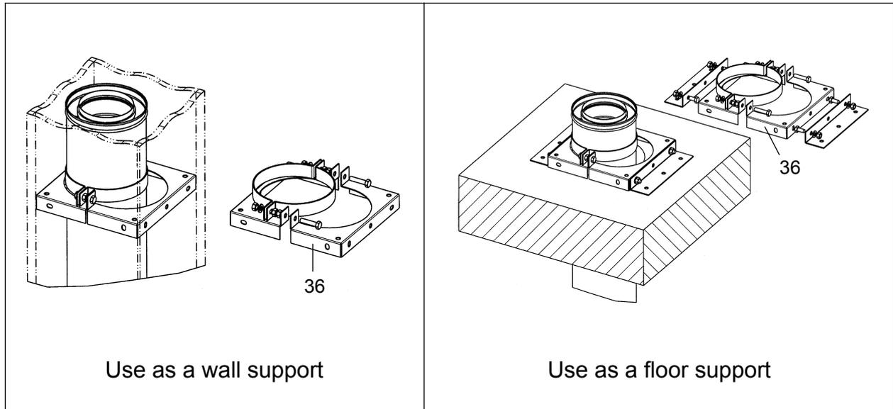
**Figure 3: Application universal wall/floor support Ø150 mm**
